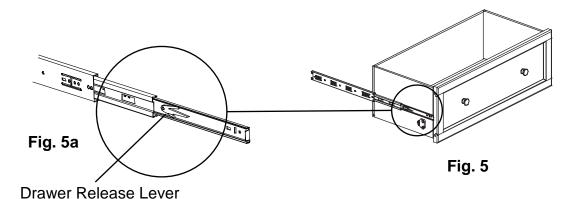
6. When removing drawers from furniture featuring the Anti-Tip Drawer Interlock System it is important that the drawer be installed back in its original location. Numbers and letters are stamped on the back of the drawers. Stamping sequence starts at the bottom, moves to the top and designated left or right.
