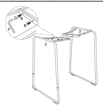
Attach the metal frame (2) to metal frame (3) by using bolts (B) and wrench (F). Do not tighten bolts completely until step #2.
