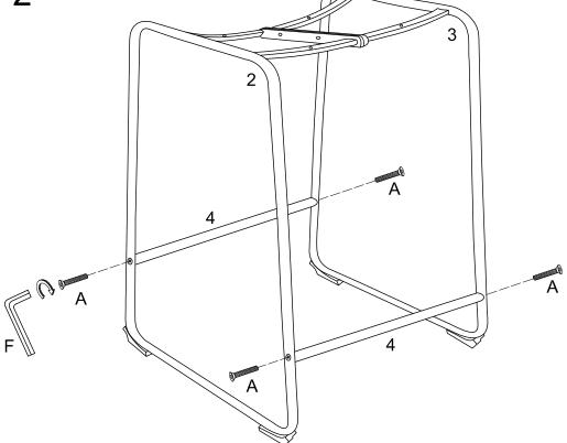
Attach the metal tubes (4) to the metal frame (2)(3) and secure it by using bolts (A) and wrench (F). Tighten bolts from assembly in Step 1.
