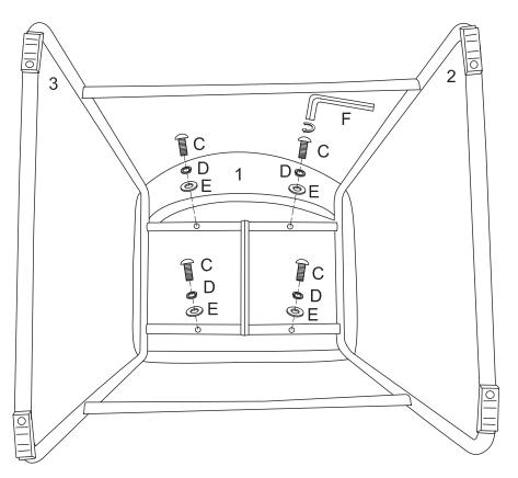
Attach the seating frame (1) to the metal frame (2)(3) and secure it by using washers (E), spring washers (D) and wrench (F).
