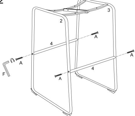
Attach the metal tubes (4) to the metal frame (2)(3) and secure it by using bolts (A) and wrench (F). Tighten bolts from assembly in Step 1.
