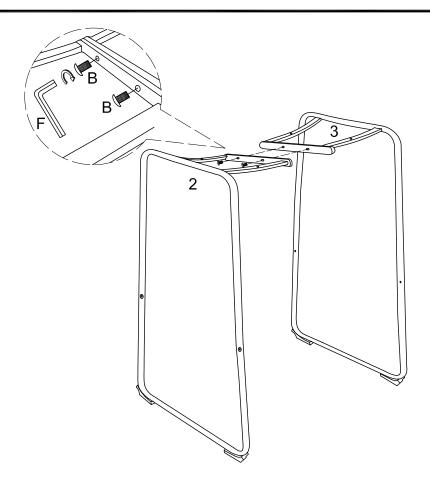
Attach the metal frame (2) to the metal frame (3) by using bolts (B) and wrench (F). Do not tighten bolts completely until step #2.
