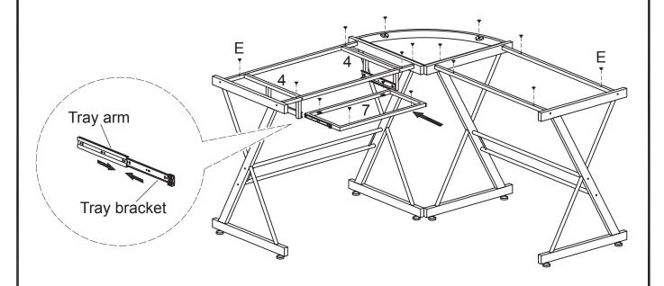
Carefully slide keyboard tray frame (7) into place. The tray brackets attached to keyboard tray frame (7) will slide into the tray arms attached to the keyboard tray supports (4). Insert rubber suction cups (E) into the desk frame as shown above.
