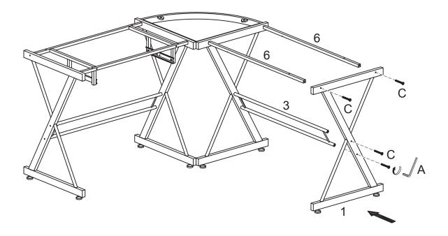
Attach leg (1) to upper crossbars (6) and lower crossbar (3) using medium bolts (C). Tighten medium bolts (C) with wrench (A).
