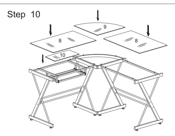
Carefully lay keyboard tray glass (10) in place and gently press to secure. Carefully lay glass (8) and corner glass (9) in place and gently press to secure.
