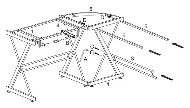
Attach the tray arms of keyboard tray sliders (G) to keyboard tray supports (4) using short bolts (B). *Ensure that the open end of each tray arm is near the front of the desk*. Tighten short bolts (B) with a screwdriver. Attach leg (1) and crossbars (6) to corner frame (5) using long bolts (D). Attach lower crossbar (3) to leg (1) using medium bolts (C). Tighten all bolts (C,D) with wrench (A).
