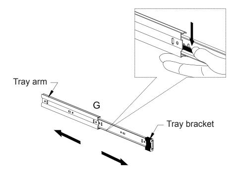
Disassemble keyboard tray slider (G) by sliding the tray arm and tray bracket apart. Depress the small lever of the tray bracket and carefully pull the two pieces apart. Repeat this process for both keyboard tray sliders (G).
