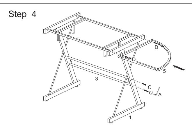
Attach leg (1) and corner frame (5) to the assembly from the previous step using long bolts (D). *Ensure that the glass supports of corner frame (5) are facing up (reference Steps 8 and 9).* Secure leg (1) to lower crossbar (3) using medium bolts (C). Tighten all bolts with wrench (A).
