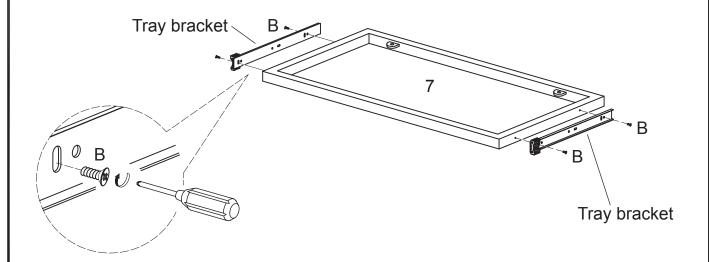
Attach the tray brackets of keyboard tray sliders (G) to keyboard tray frame (7) using short bolts (B). Ensure that the open end of each tray bracket is near the back of keyboard tray frame (7). Tighten short bolts (B) with a screwdriver.
