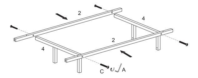
Attach upper crossbars (2) to keyboard tray supports (4) using medium bolts (C). *Note the proper alignment of all bolt holes as shown above.* Tighten medium bolts (C) with wrench (A).
