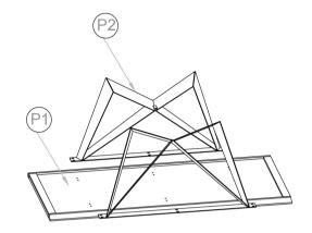
**STEP 2.** First attach the leg's using Allen Bolt with the help of Allen Key as shown in fig. (do not screw tight), then attach the legs with the Top as shown in fig.
