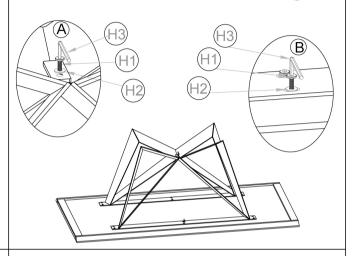
**STEP 3.** Now fully tight the legs using Allen Bolt with the help of Allen Key.
