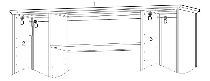
Secure top panel (1) to panels (2,3) using cam locks (D). Tighten cam locks (D) with a screwdriver.
