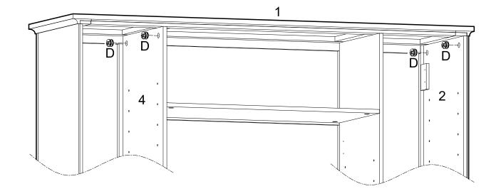
Secure top panel (1) to panels (2,4) using cam locks (D). Tighten cam locks (D) with a screwdriver.
