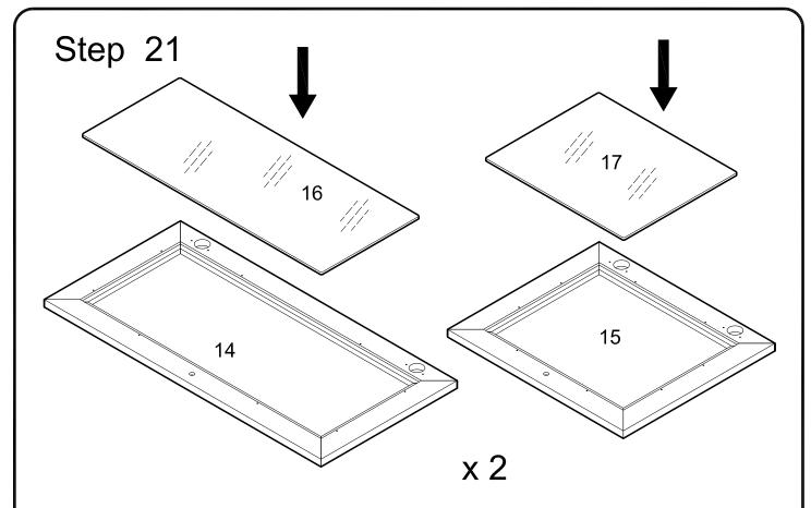
Carefully lay glass panel (16) into door (14) and glass panel (17) into door (15). Repeat this step for the second set of glass panels and doors.
