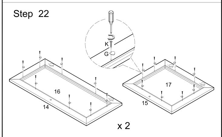
Secure glass panel (16) to door (14) and glass panel (17) to door (15) and secure it with the metal washers (G) and screws (K).
