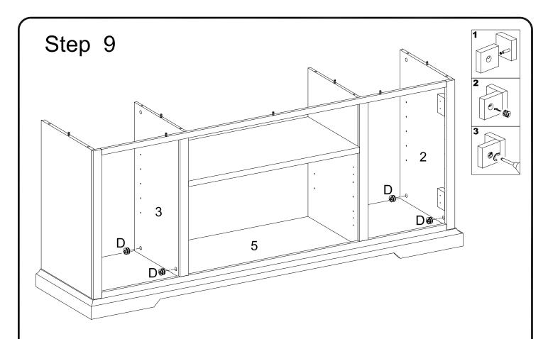
Secure panels (2,3) to bottom panel (5) using cam locks (D). Tighten cam locks (D) with a screwdriver.
