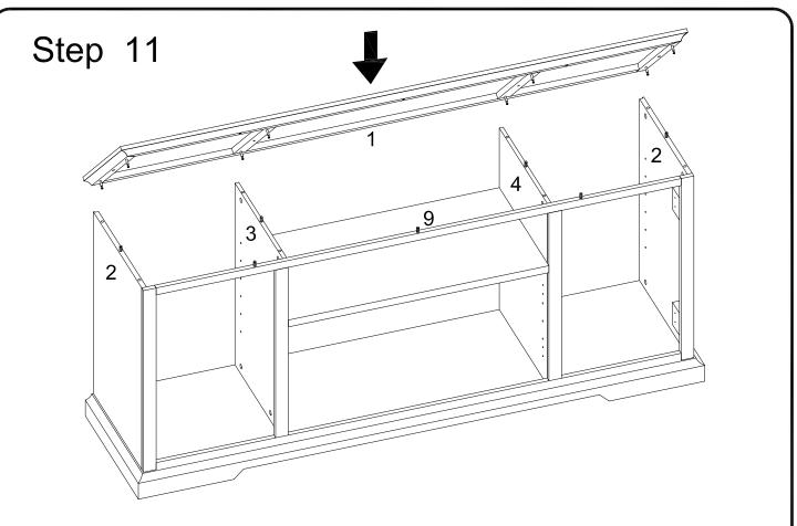
Carefully fit top panel (1) into place using cam bolts and dowels as guides.
