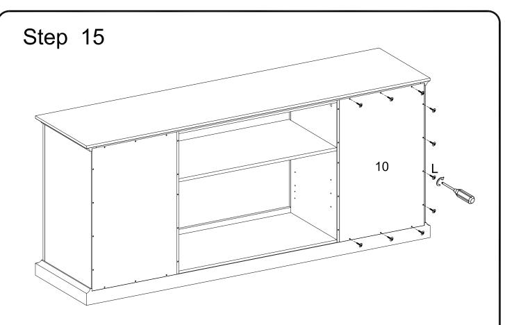
Attach panel (10) to the back of the console using screws (L).
