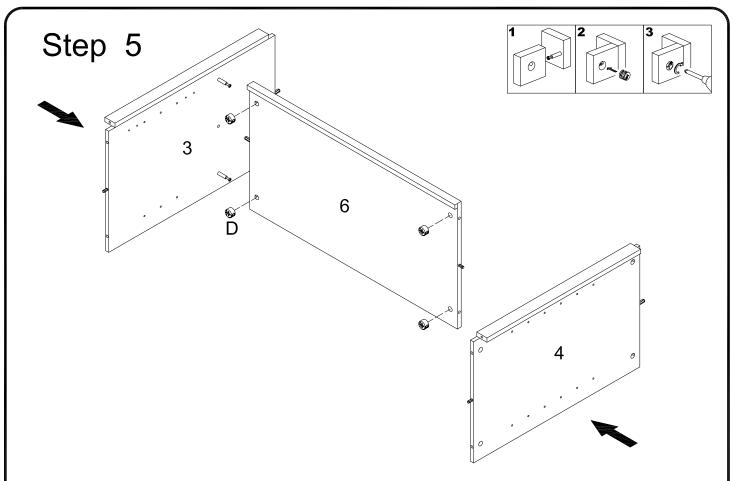
Attach panels (3,4) to panel (6) using cam bolts and dowels as guides. Secure panels (3,4) t panel (6) using cam locks (D). Tighten cam locks (D) with a screwdriver.
