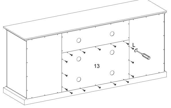
Attach panel (13) to the back of the console using screws (L).
