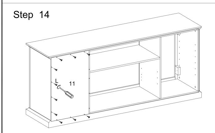
Attach panel (11) to the back of the console using screw (L).
