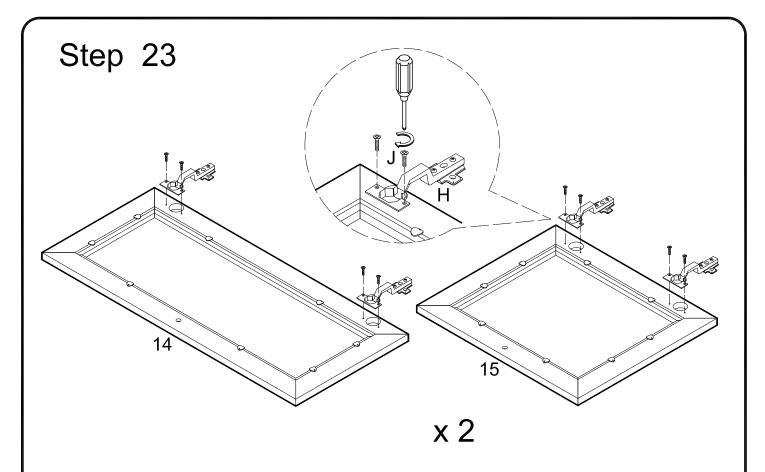
Attach hinges (H) to door (14,15) using screws (J). Repeat this step for the second set of doors.
