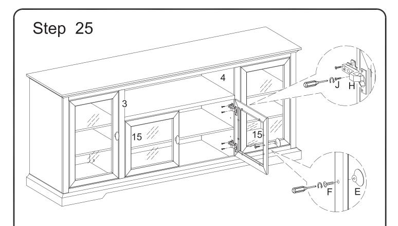
Attach doors (15) to panels (3,4) using screws (J) at hinges (H). See page 2 for specific instructions on how to adjust hinges so doors are aligned with console as desired. Attach handles (E) to doors (15) using bolts (F).
