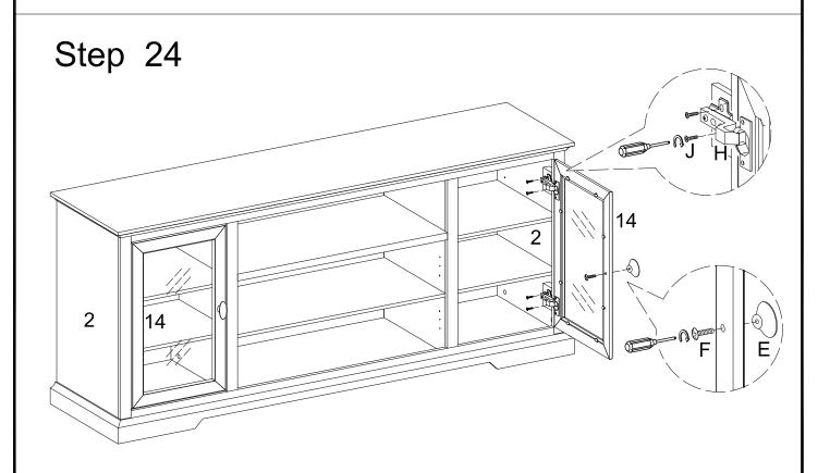
Attach doors (14) to panels (2) using screws (J) at hinges (H). See page 2 for specific instructions on how to adjust hinges so doors are aligned with console as desired. Attach handles (E) to doors (14) using bolts (F).
