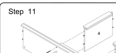
Assemble the side panel (4,5) to the bottom panel (2) and secure it by bolt (D) and wrench (L).
