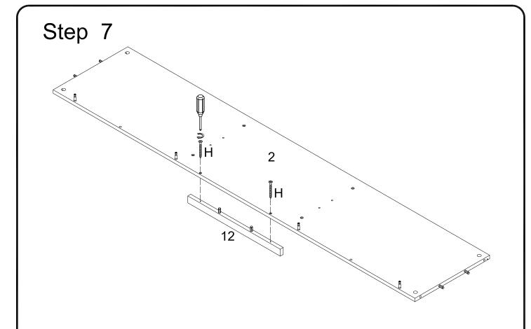
Upside down the bottom panel (2) and assemble the front panel (12) with screw (H).
