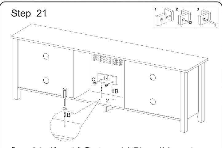
For security, insert the cam bolts (B) and use cam lock (C) to assemble the support panel (14) to the bottom panel (2).
