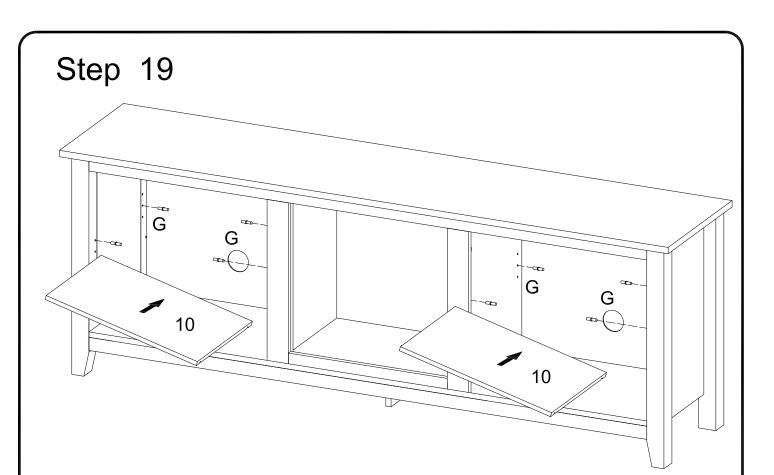
Input the shelf support pin (G) to the stand and place the wooden shelf (10) on top.
