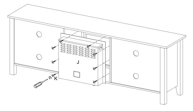
Assemble the fireplace insert (J) to the stand and secure it with screw (K).
