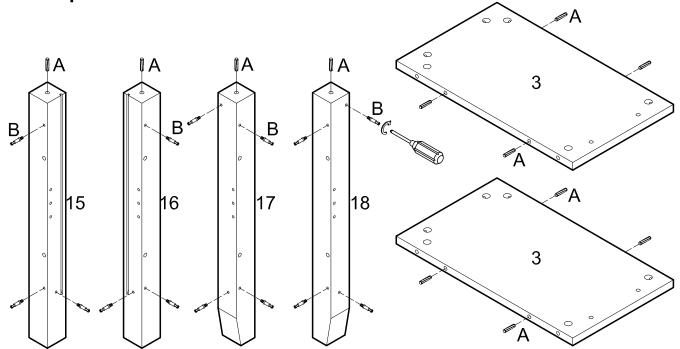
Insert the wooden dowel (A), cam bolt (B) into the wooden legs (15,16,17,18). Insert the wooden dowel (A) into the side panel (3).
