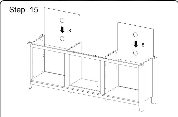
Right up the stand and slot in the back panel (8) to the side panels. Please pay attention on the corner direction of the back panel.
