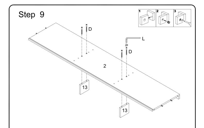
Attach support legs (13) to panel (2) using bolts (D). Tighten bolts (D) with wrench (L).
