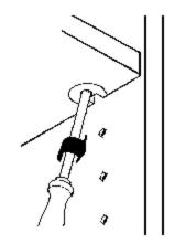
Position the screwdriver at a 25° angle.
