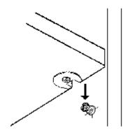
4. Using a Phillips Screwdriver at a 25° angle, tighten the Cam about a half turn.
