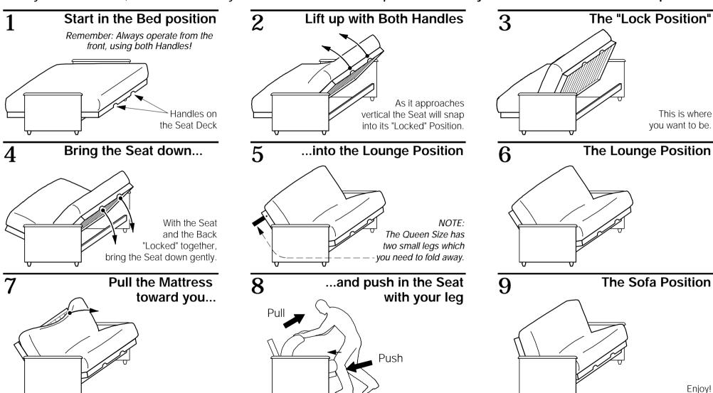
Please Note: If the rollers of the mechanism become improperly disengaged, the Back Deck could come down more quickly than you expect!
